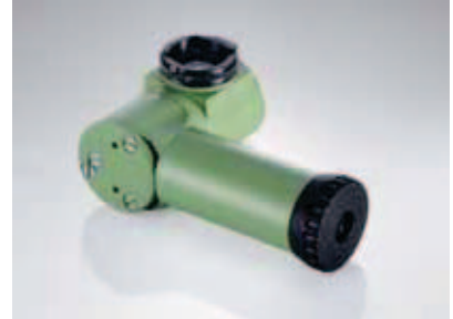
GOK6, Diagonal Eyepiece For comfortable observations of steep sights, up to 66°. Has a variable joint for the adjusting the sighting angle. Fits all TPS instruments. Includes objective counterweight. Order No: 376 236
